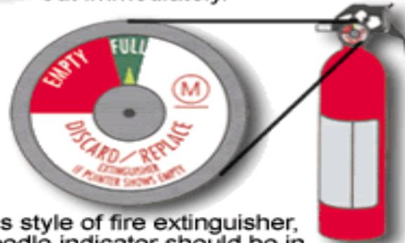
On this style of fire extinguisher, the needle indicator should be in the "full" range.
