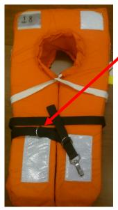
Recent Coast Guard inspections of Type I Personal Flotation Devices, (PFDs) in both adult and child size, identified a potential hazard that could prevent proper donning in the event of an emergency. The chest strap was threaded through the fixed "D" ring that the strap is intended to clip to when worn. (Image left)
