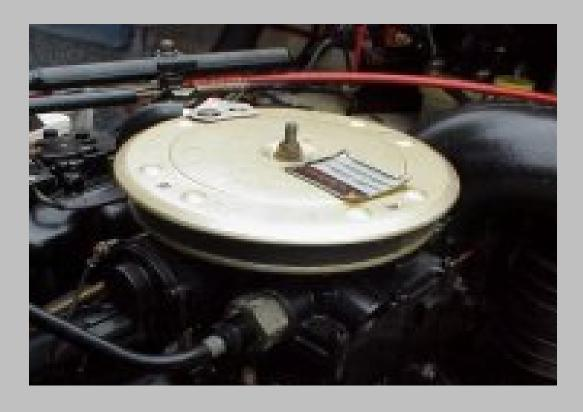
All gasoline powered inboard/outboard or inboard motor boats must be equipped with an approved backfire
